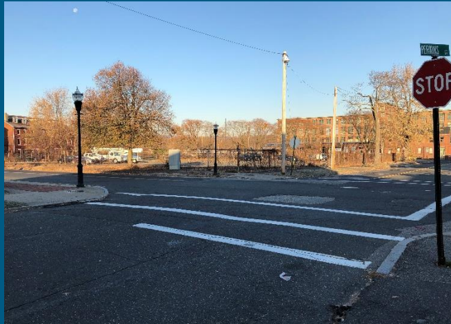
Poor pedestrian conditions at Exchange Street at Perkins Street due to lack of accessible curb ramps, unmarked crossings, and poor sidewalk conditions with obstructions.
